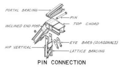
Figure 5: Structural Components (from PennDOT Truss Maintenance Manual, 2015)
